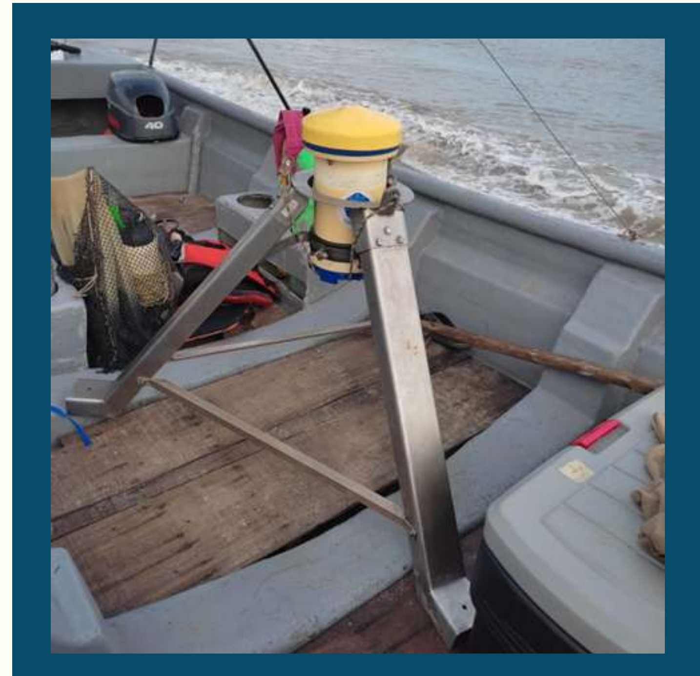
(a) Location of measuring points with ADCP and bathymetric profile. (b) Boat with support structure for the ADCP
