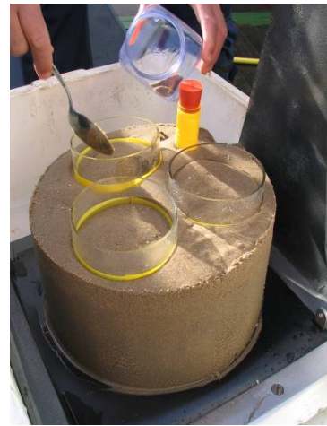
Fig.4. Boxcore sample (0.07 m 2 ; ~20 cm deep) with 3 sub-cores (diam. 10 cm; 0.024 m 2 total surface) inserted 5 cm deep for sampling juvenile bivalves. The smaller fourth core is for collection of sediment.
