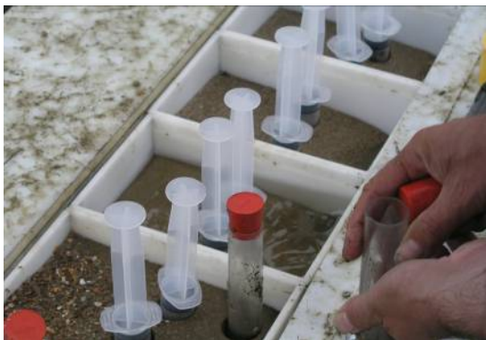
Fig. 9. Mesocosms with different sand fractions: (a) each lander contained 3 mesocosm trays containing 6 small boxes and closing lids; (b) each mesocosm tray contained 6 settlement boxes filled with different types of sediment; (c) sub samples were taken with small cores for juvenile benthos and with syringes to collect sediment.
