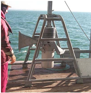
Fig. 3. Reineck boxcorer (sample size 0.07 m 2 ) for sampling in- and epifauna.
