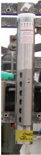
Fig. 8. Seabird 37-SPM Microcat for recording conductivity and temperature.
