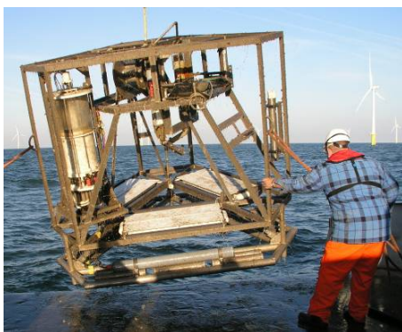
Fig. 5. Lander with autonomous sensors and mesocosms ready for deploy.
