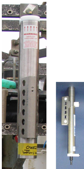
Fig. 8. Seabird 37-SPM Microcat for recording of conductivity and temperature.
