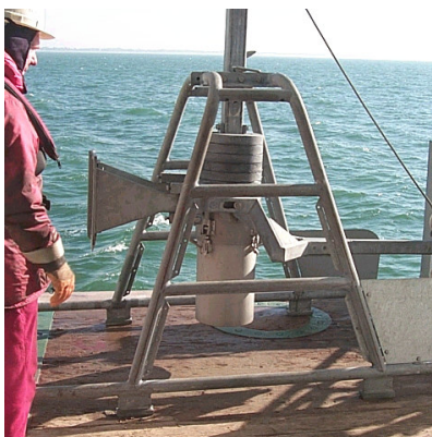
Fig. 3. Reineck boxcore (sample size 0.07 m 2 ) for sampling in- and epifauna.
