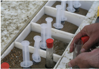
Fig. 9. Mesocosms with manipulated sediments; a. each lander contained 3 mesocosm trays with lids; b. each mesocosm tray contained 6 settlement boxes; c. sub samples were taken with small cores for juvenile benthos and with syringes to collect sediment.
