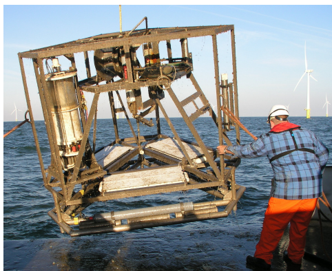
Fig. 5. Lander with autonomous sensors and experimental mesocosms ready for deploy.
