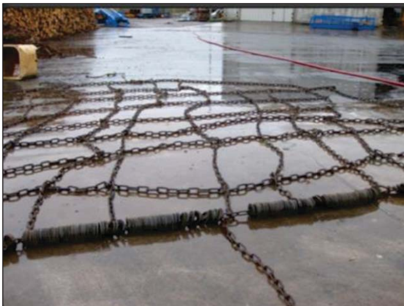
Figure 8-1: Photograph showing a chain mat using for trawl sweeps (courtesy of SFF).
