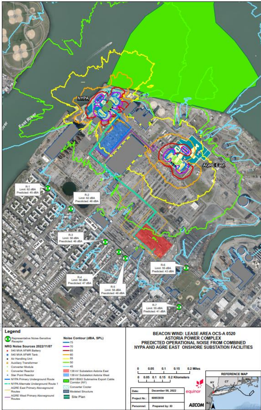
FIGURE 4.4-14. PREDICTED NOISE CONTOURS FOR BOTH NYPA AND AGRE EAST ONSHORE SUBSTATION FACILITIES
