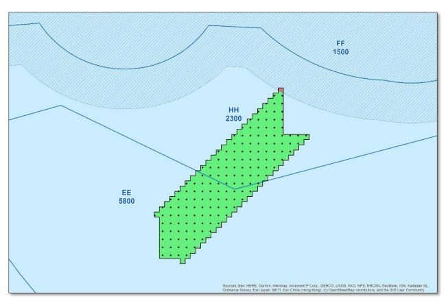
Figure 10: Boston Consolidated (A90) TRACON FUSION 5 MVA sectors (blue) with Sector FF obstacle evaluation area (hatched blue)
