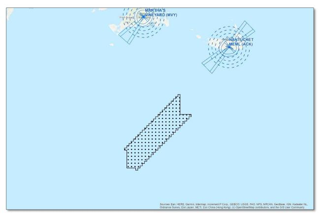
Figure 3: 14 CFR Part 77.17(a)(2) obstruction standard (dashed blue) and 77.19 (solid blue) imaginary surfaces in proximity to the Beacon Wind project
