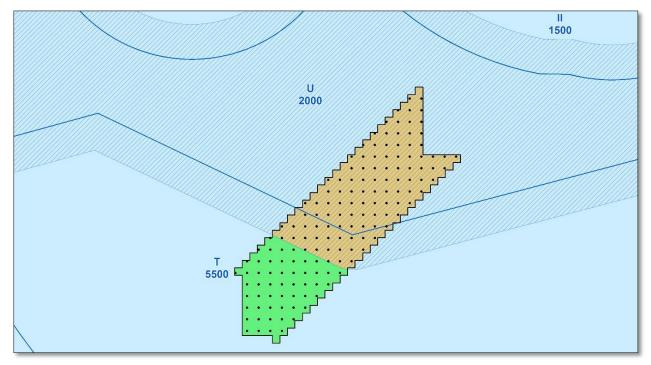
Figure 9: Boston Consolidated (A90) TRACON FUSION 3 MVA sectors (blue) with Sector U obstacle evaluation area (hatched blue)
