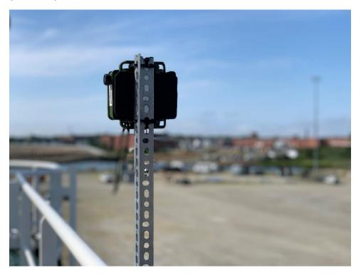
PHOTOGRAPH 2. INSTALLATION OF BAT DETECTOR ON STARBOARD SIDE OF *STRIL EXPLORER* BRIDGE (HANDRAIL). AUGUST 9, 2020.
