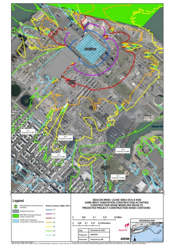
FIGURE K.5-10. PREDICTED NOISE CONTOURS FOR SUBSTATION CONSTRUCTION ACTIVITIES AT AGRE WEST
