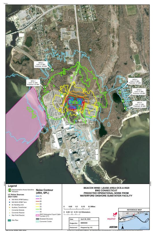
FIGURE K.5-5. PREDICTED NOISE CONTOURS FOR THE ONSHORE SUBSTATION FACILITY AT WATERFORD, CONNECTICUT
