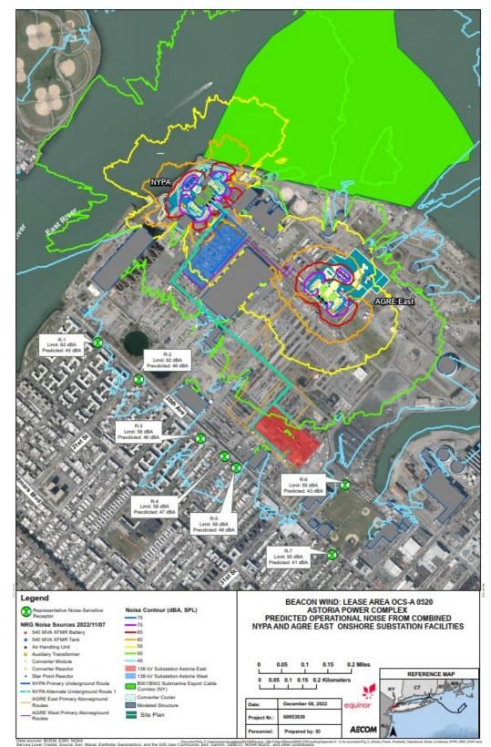
FIGURE K.5-4. PREDICTED NOISE CONTOURS FOR THE COMBINED ONSHORE SUBSTATION FACILITIES AT NYPA AND AGRE EAST
