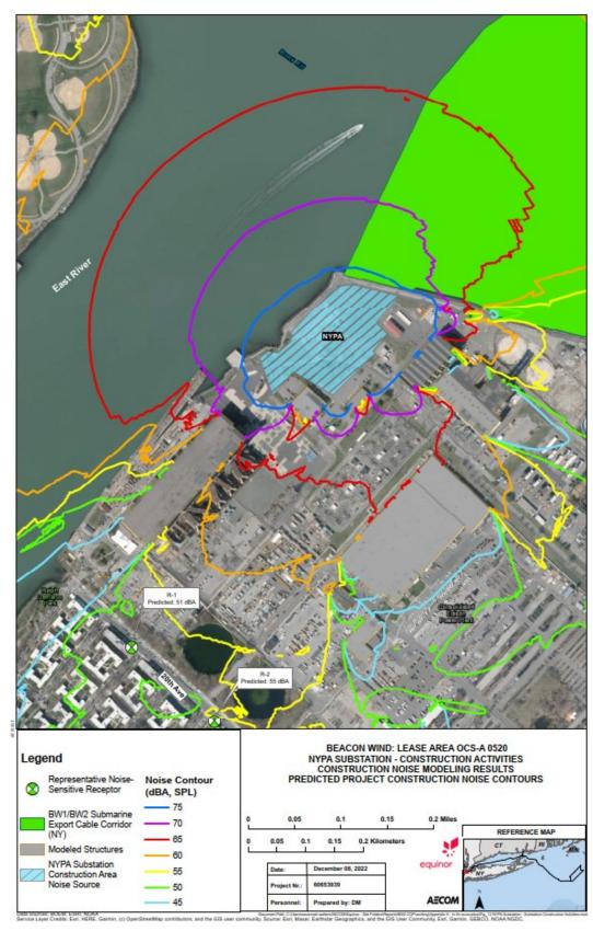
FIGURE K.5-9. PREDICTED NOISE CONTOURS FOR SUBSTATION CONSTRUCTION ACTIVITIES AT NYPA
