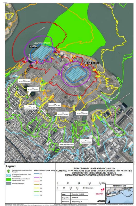
FIGURE K.5-12. PREDICTED NOISE CONTOURS FOR COMBINED SUBSTATION CONSTRUCTION ACTIVITIES AT NYPA AND AGRE EAST
