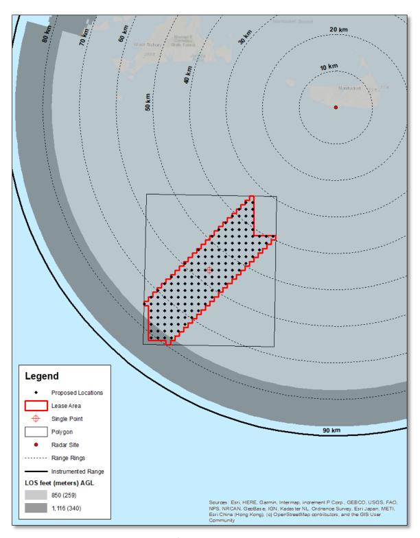
Figure 17 LOS Analysis Results for the Nantucket HF Radar using 10-meter NED
