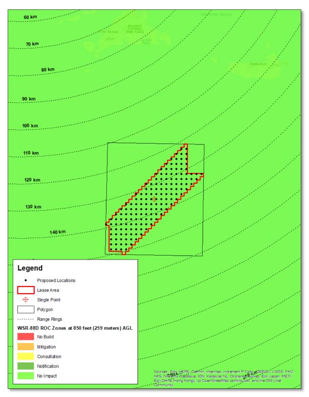
Figure 6 WSR-88D ROC Zone Results at 850 feet (259 meters) AGL for the Boston WSR-88D using 10-meter NED
