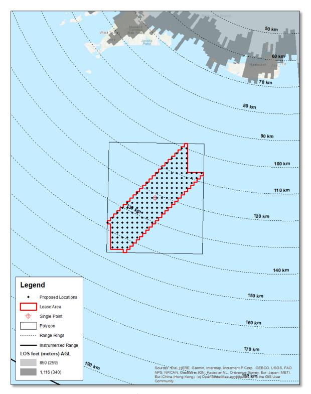
Figure 19 LOS Analysis Results for the Nauset HF Radar using 10-meter NED
