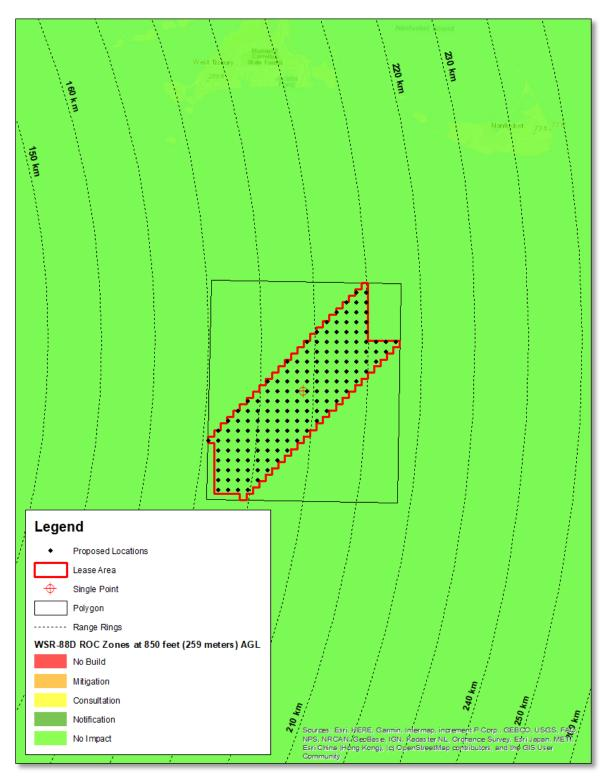
Figure 8 WSR-88D ROC Zone Results at 850 feet (259 meters) AGL for the Brookhaven WSR-88D using 10-meter NED
