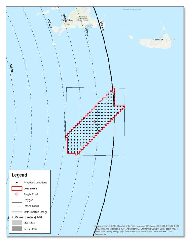
Figure 15 LOS Analysis Results for the Moriches HF Radar using 10-meter NED
