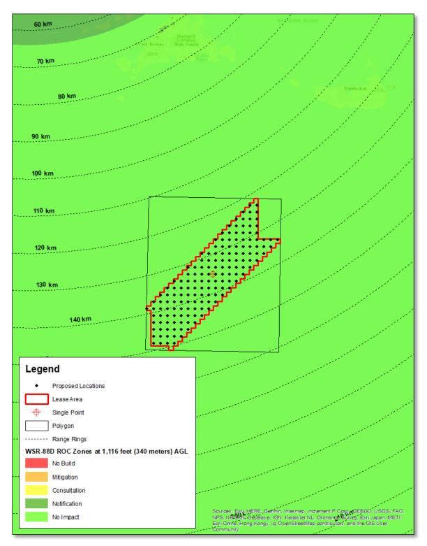
Figure 7 WSR-88D ROC Zone Results at 1,116 feet (340 meters) AGL for the Boston WSR-88D using 10-meter NED
