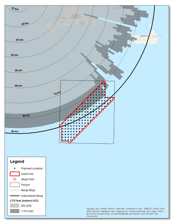
Figure 12 LOS Analysis Results for the Horseneck Beach State Reservation HF Radar using 10-meter NED
