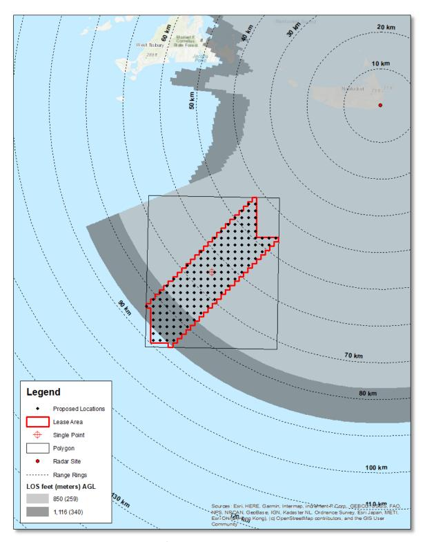
Figure 18 LOS Analysis Results for the Nantucket Island HF Radar using 10-meter NED
