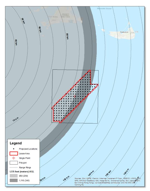
Figure 11 LOS Analysis Results for the Block Island Long Range HF Radar using 10-meter NED
