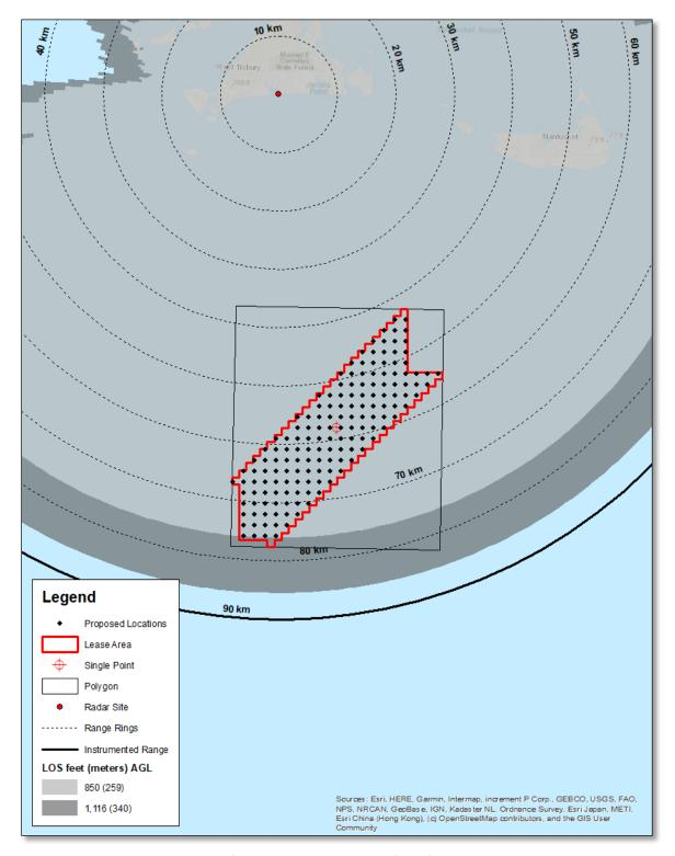
Figure 13 LOS Analysis Results for the Long Point Wildlife Refuge HF Radar using 10-meter NED
