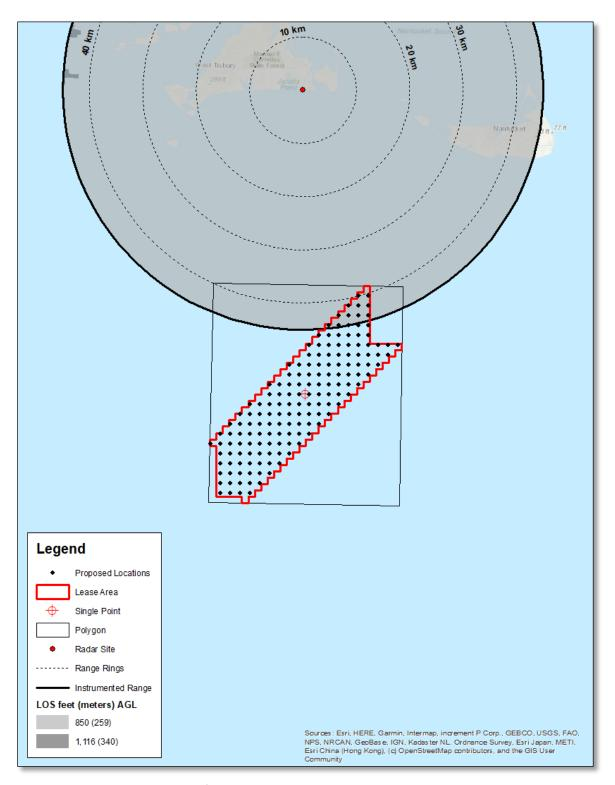
Figure 16 LOS Analysis Results for the MVCO Meteorological Mast HF Radar using 10-meter NED
