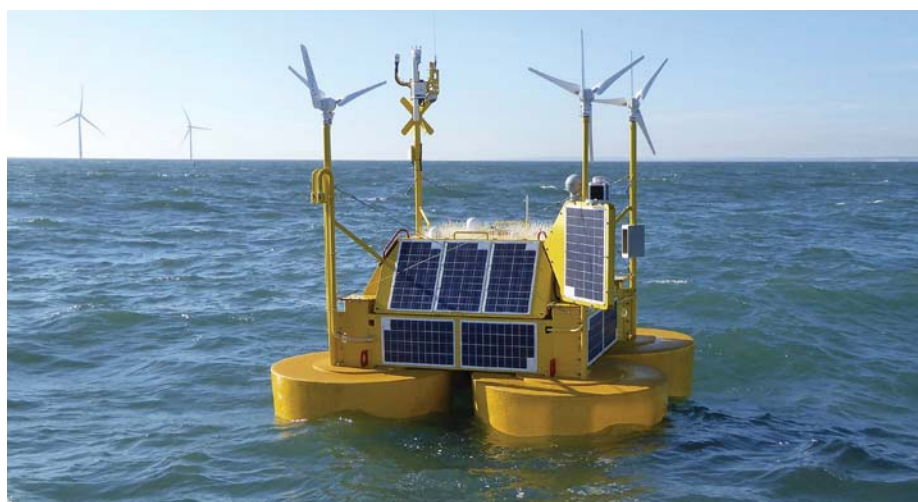
FIGURE 2. In 2019, the New York State Energy Research and Development Authority commissioned the deployment of two floating lidar buoys in the New York Bight. These buoy-based lidars provided nearly three years of physical metoccean parameters to facilitate offshore wind development within the region. Parameters include multi-level wind speed and direction, wave, and current measurements, as well as other environmental and wildlife data. Courtesy of New York State Energy Research and Development Authority, https://oswbuoysny.resourcepanorama.dnvgl.com/overview
