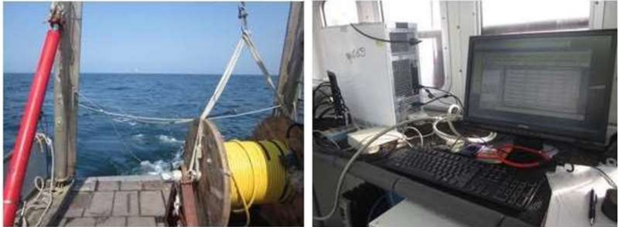
Figure 12. The left photo shows the towed array trailing aft of the Research Vessel Shanna Rose and the data collection equipment in the lab of the vessel is shown on the right photo.
