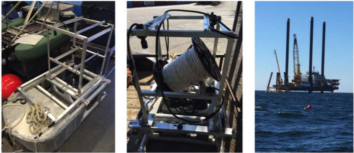
Figure 17. (Left and Center) Images of the geophysical sled before deployment. These two photos show the tetrahedral array of hydrophones with a spacing of 0.5 m. (Right) photo of the surface floats for the sled with WTG#4 in the background.
