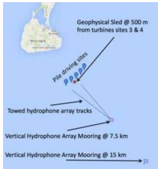
Figure 10. Locations of the Geophysical Sled 500 meters from wind turbines 3 and 4, the Vertical Hydrophone Arrays at 7.5 and 15 km distance and the Towed Hydrophone Array tracks.
