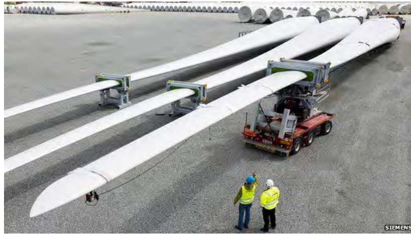
Figure 4-11. Example of specialized upland equipment to maneuver blades (Siemens 2014)
