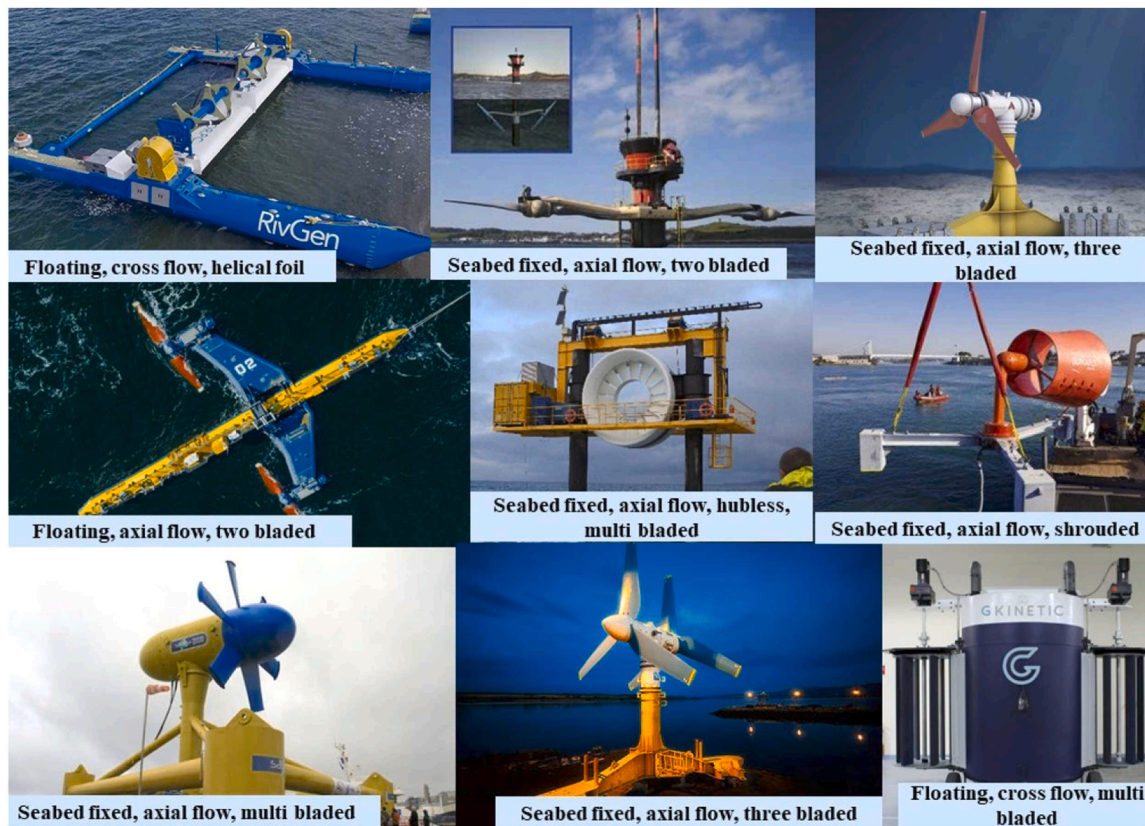
Fig. 2. Diversity of tidal stream devices' configurations (Munaweera Thanthirige et al., 2025).
