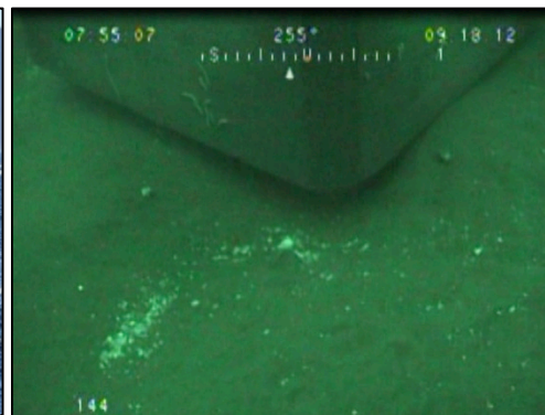
L: The Ocean Sentinel deployed at the test site just north of Yaquina Head Newport, OR R: Scour undercutting sediment under the concrete anchor and accumulation of shell hash
