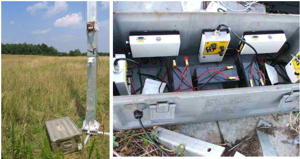
Figure 5. Military surplus dry boxes used to store acoustic detectors at ground-level during the study.
