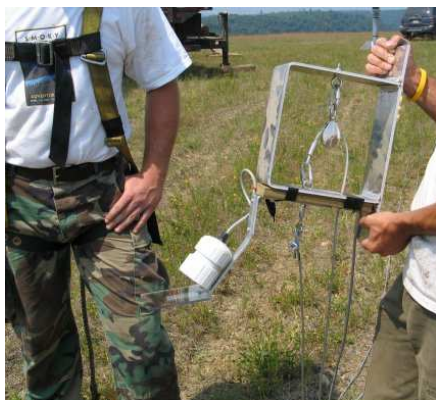
A. Pulley system for deploying “bat hats.”
