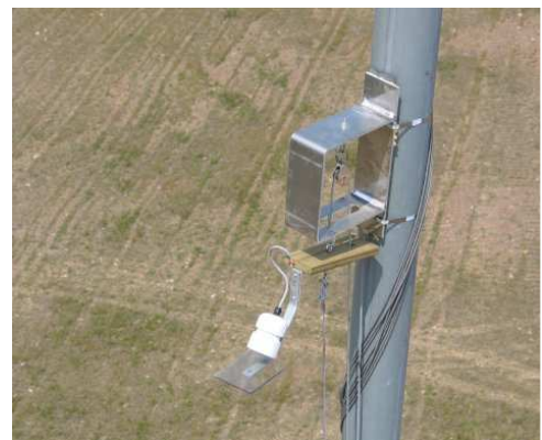
C. A mounted pulley system and bat hat at 22 m high.
