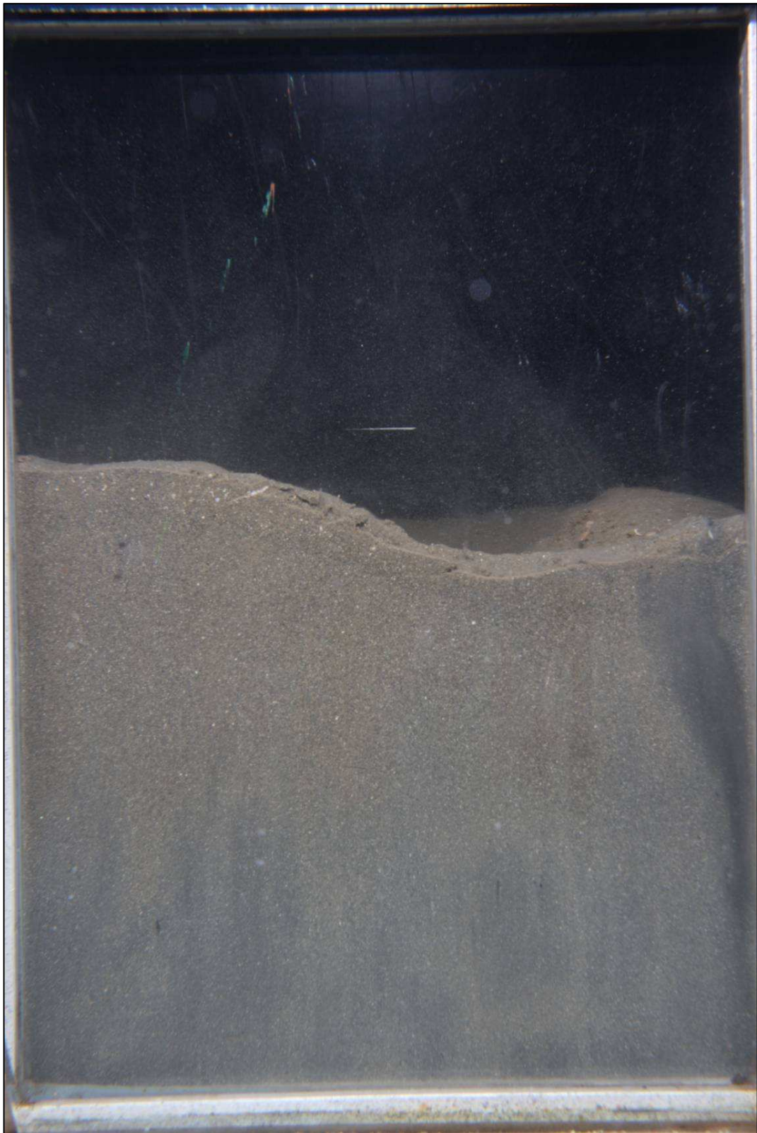
Figure 1: SPI image at ocean energy device site showing well oxygenated sediment with biologically generated surface boundary roughness.
