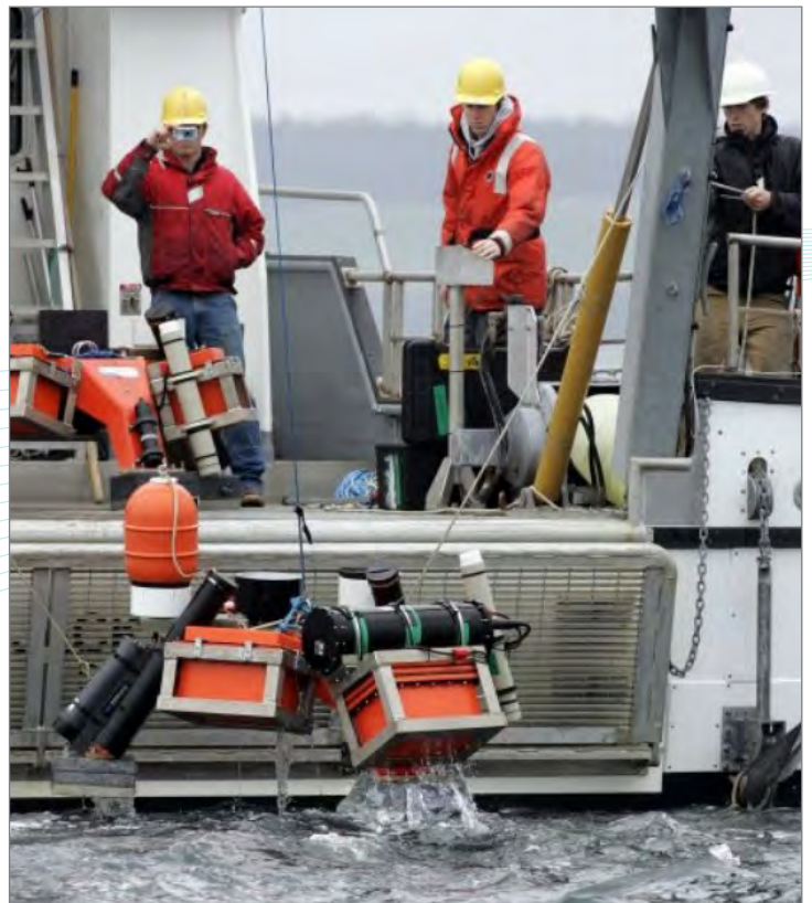
Fully rigged DT-X SUB as deployed for 5-week seafloor observatory mission.
