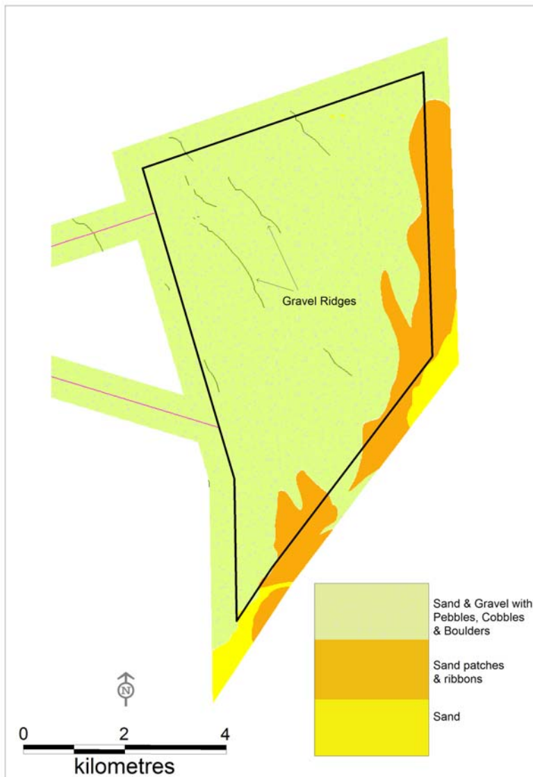
Figure 2. Seabed Features of proposed wind farm site from geophysical survey.
