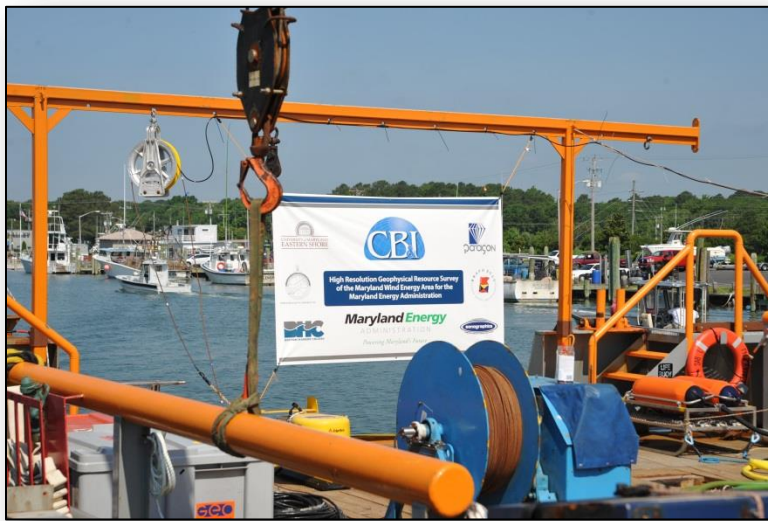
Figure 5: Back deck and "H" frame of the m/v Scarlett Isabella in Ocean City, Maryland during mobilization. Oceanographic winch, sparker sled, and chirp towfish can all be seen on deck.
