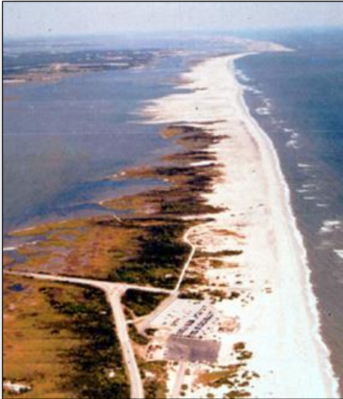
Figure 4: Aerial Photograph looking north from Assateague Island toward Ocean City. This image shows erosion at the northern part of the island (south of the Ocean City Inlet), contributing to the appearance of landward migration (Zimmerman, 2000).
