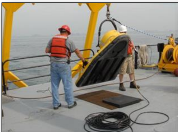
Figure 15: Image of the sub-bottom profiler 512i towfish used in the MEA HRG.
