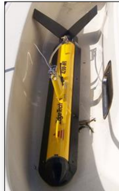
Figure 13: Image of the EdgeTech 4200 Sidescan Sonar towfish used in the MEA HRG.
