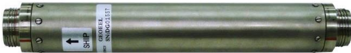
Figure 19: GeoEel analog to digital (A/D) converter module.
