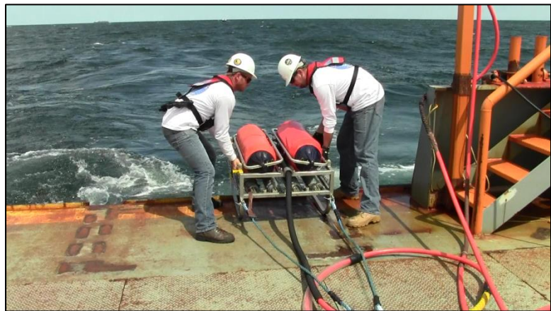
Figure 7: Jeff Helgerson (L) and Chris Dougherty (R) deploying the sparker sound source sled from the stern of the m/v Scarlett Isabella in the Maryland WEA.
