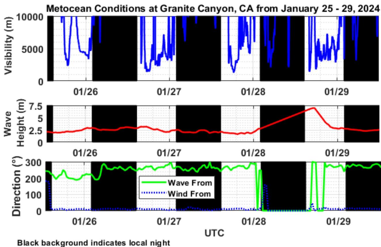
**Fig. 2** Visibility was measured with a surface-based Campbell Scientific CS120A visibility sensor and typically decreased during daylight hours
