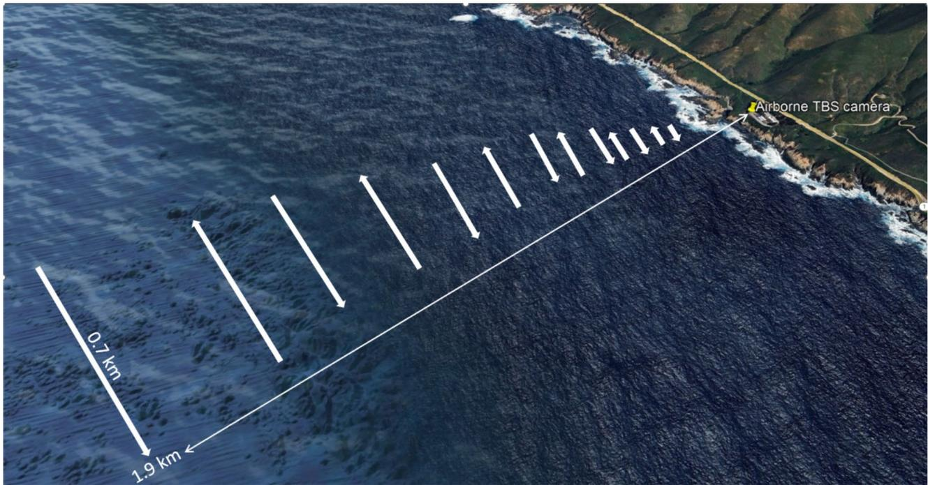
**Fig. 6** Depiction of a variable-pitch scan at a TBS altitude of 100 m agl. The direction of an arrow indicates the direction of a scan
