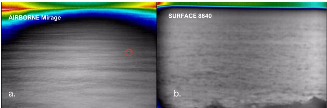
**Fig. 11** (a) The airborne Mirage sensor detection of a whale blow (red circle). (b) The detection is not visible in the surface 8640 camera image
