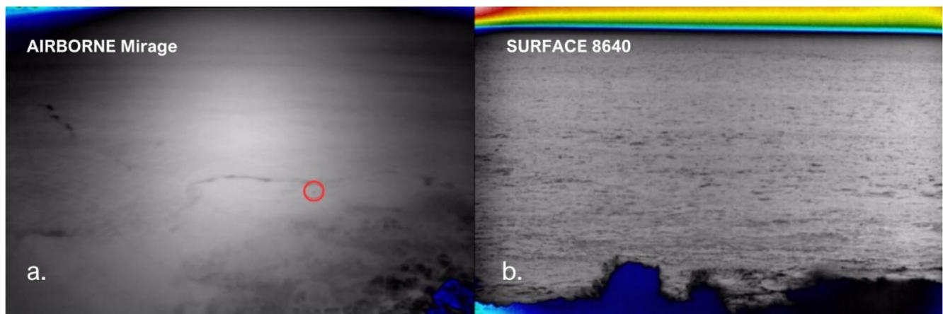
**Fig. 12** (a) An airborne avian detection by the Mirage sensor, circled in red. (b) The detection is not shown in the 8640 simultaneous sensor image because the target was beyond the field of view
