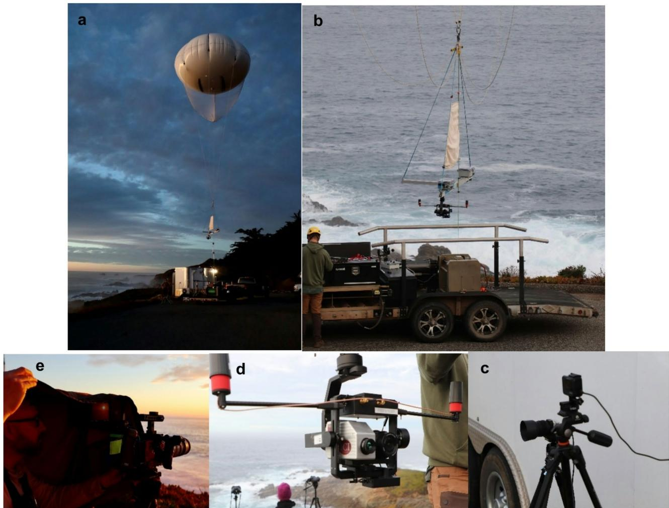
**Fig. 4** Clockwise from top left: (a) The airborne camera boom launching on the TBS; (b) the camera boom, suspended gimbal, and GNSS differential antennas above the TBS winch; (c) the ICI 8640 camera continuously operated at the surface from January 27 to January 30;
