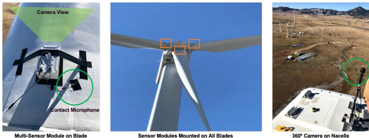
**Figure 15.** Installation of multi-sensor modules and contact microphones on each blade of a GE 1.5MW wind turbine for collision detection and image capture, and a 360° camera installed on the nacelle roof for eagle detection.
