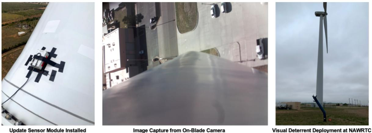
**Figure 22.** Installation and verification of system components on a 1.5MW GE wind turbine at NAWRTC, Mesalands Community College, Tucumcari, NM.
