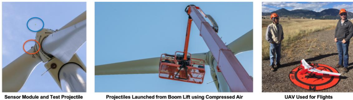
**Figure 28.** Data collection includes surrogate blade strikes using projectiles (tennis balls and potatoes), as well as programmed fixed-wing UAV flights for recording 360° and high-resolution video images from the nacelle.
