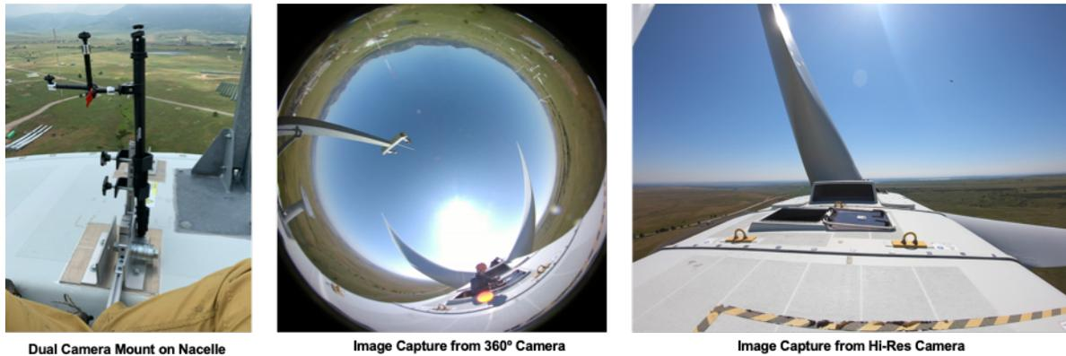
**Figure 27.** Installation and of final nacelle system components on a 1.5MW GE wind turbine at NREL-NWTC in Boulder, CO providing both 360° camera and high-resolution camera images and video for testing.
