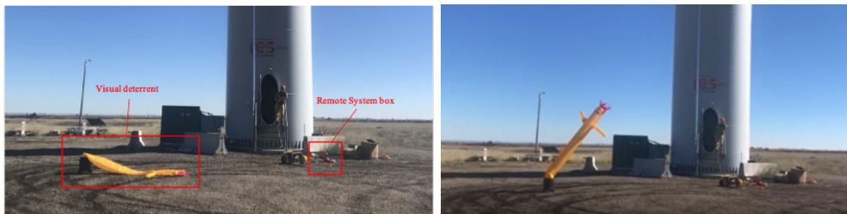
**Figure 16.** Installation and testing of visual deterrent near the base of the 1.5MW wind turbine. The deterrent is activated by an artificial stimulus; in practice, this would be triggered by the eagle detection system (Task 1.00) if eagles were detected in the 360° camera video stream from the nacelle roof.
