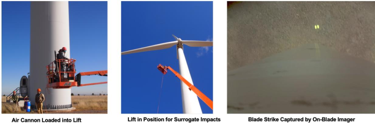
**Figure 20.** Surrogate blade strikes were conducted using soft projectiles fired at the blade using compressed air. Shown at right is an image of two tennis balls just after striking the blade, captured automatically by the on-blade collision detection module.
