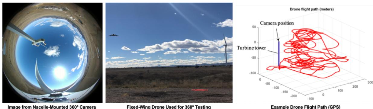
**Figure 17.** Sample image from nacelle-mounted 360° 4K camera (left); fixed-wing drone used for programmed flights and 360° capture (middle); and, GPS recording of drone flight relative to the wind turbine and camera position (right).
