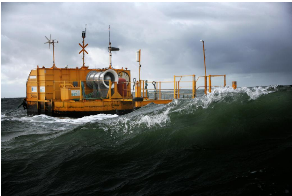
Figure4-16 : Quarter scale Ocean Energy OWC device
