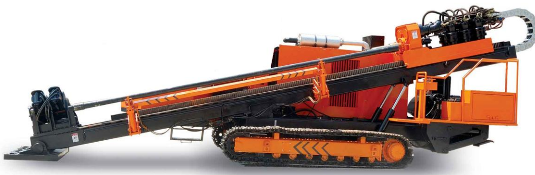
Figure 4-22: Typical horizontal directional drill
