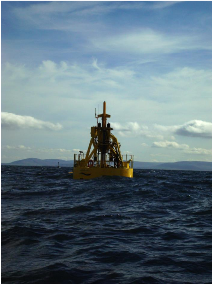
Figure 4-15: Quarter scale Wavebob WAB-PA device
