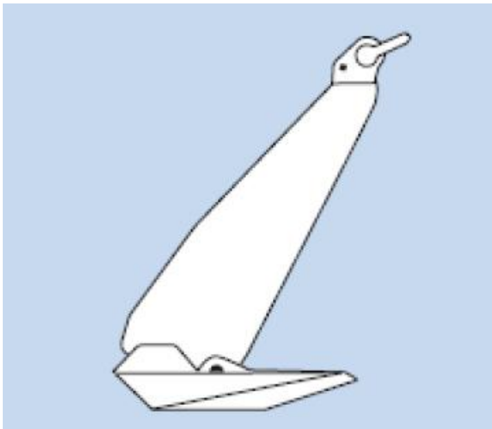
Figure 4-31: Sketch of a drag embedment anchor
