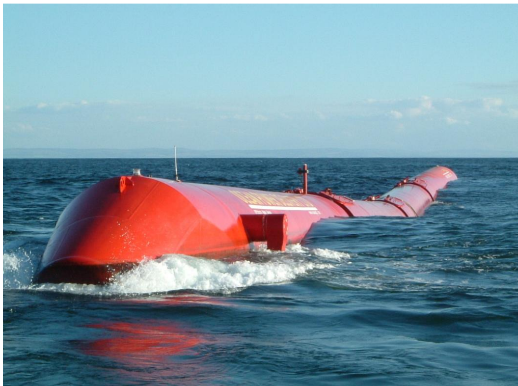
Figure 4-17: Full scale Pelamis deployment WAB-A device
