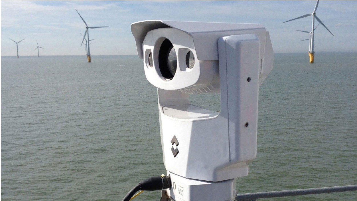
Figure 15. Thermal camera mounted on an offshore wind turbine to detect birds. Photo credit: Vattenfall.
