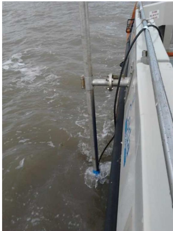
Figure 4.2: Sontek ADCP unit mounted on a swing arm during the survey (Guo et al., 2020).
