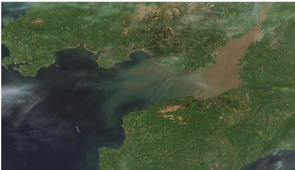
Figure 6.35: Distribution of suspended sediments in Bristol Channel and Severn Estuary observed from a satellite image (Parsons Brinckerhoff Ltd, 2010).
