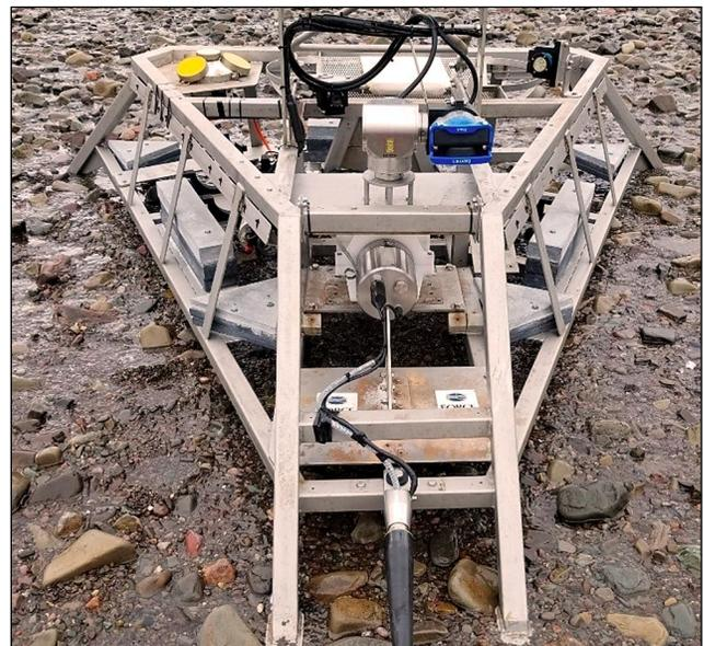
**Figure 10.11.** Fundy Ocean Research Centre for Energy (FORCE)'s Fundy Advanced Sensor Technology Environmental Monitoring System (FAST-EMS) integrated and cabled monitoring platform positioned on the FORCE beach. (Photo courtesy of FORCE)
