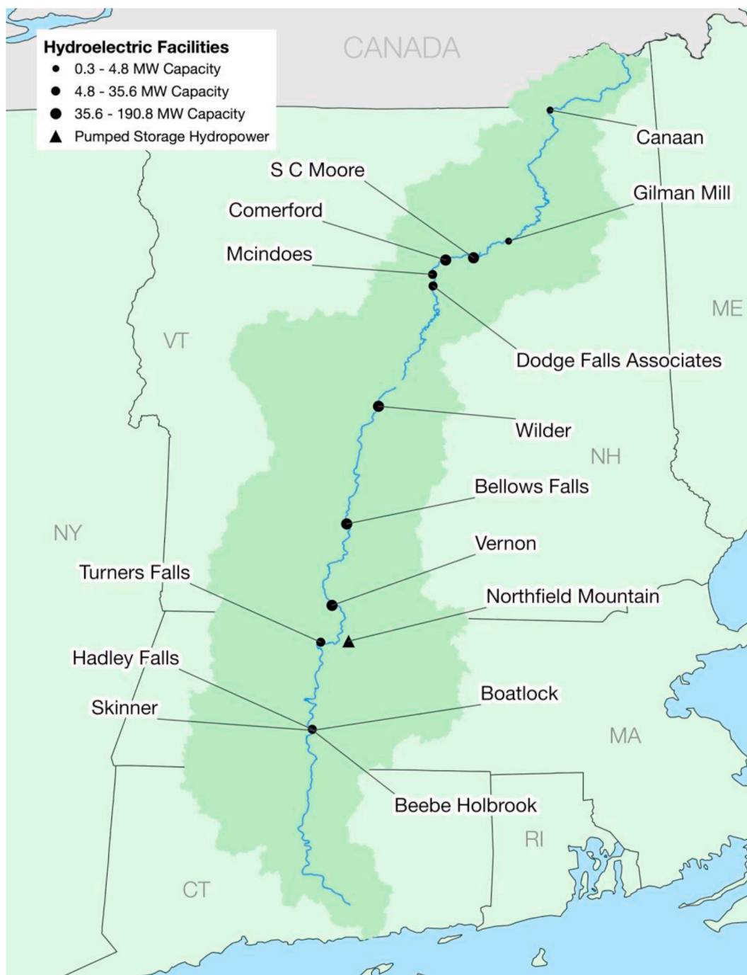
Fig. 1. Map of Connecticut River hydroelectric facilities. See Appendix, Section C for tabular data.
