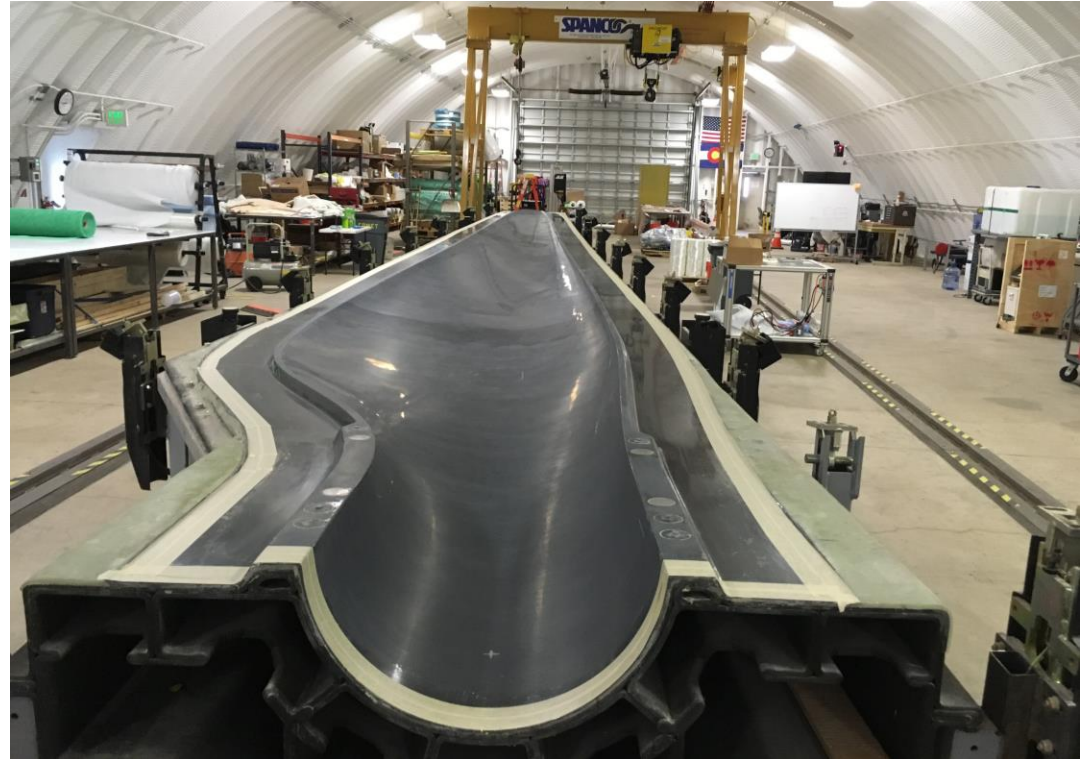
13 m blade mold printed by Oak Ridge National Laboratory
