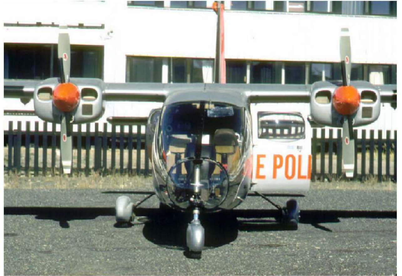
Figure 1. Partenavia P-68 Observer aircraft. Note the plexiglass nose for pilot and front seat observer, and bubble windows on both sides of the aircraft in the rear passenger panels (see on open door to right).
