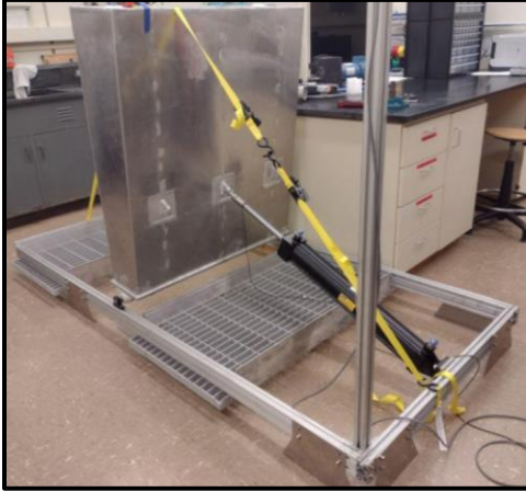
HMEC 1m x 1m oscillating surge wave energy converter (OSWEC)
