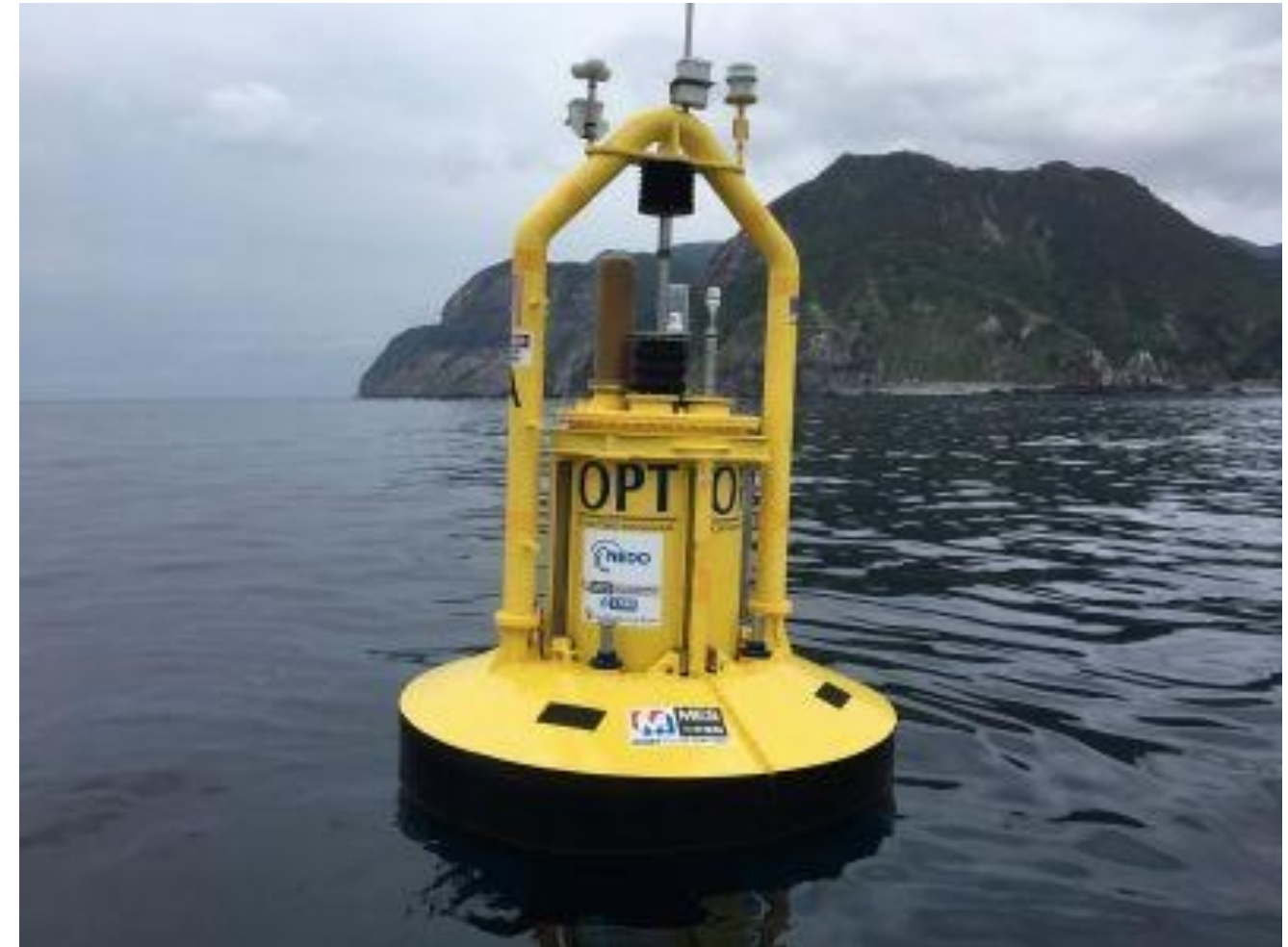
Example of a point absorber WEC: Ocean Power Technologies
