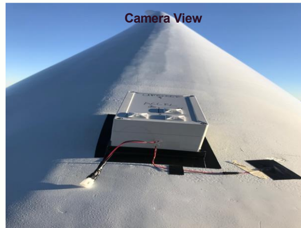
On-blade impact detection
