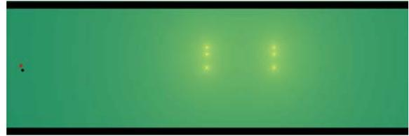
**Figure 2: Turbine layout for tidal channel scenario. Background colour indicates device/ambient sound level. The points at the left are the start locations of the two animals.**
