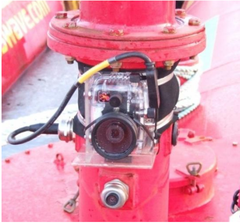
Figure 1. Autonomous stills camera mounted on the P2 machine.
