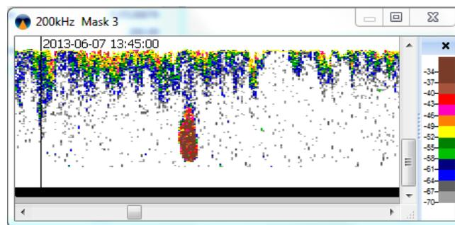
Figure 2. Echogram showing fish school highlighted as spike below "X" marked in Figure 1. Data from 200kHz transducer and scale in relative dB.
