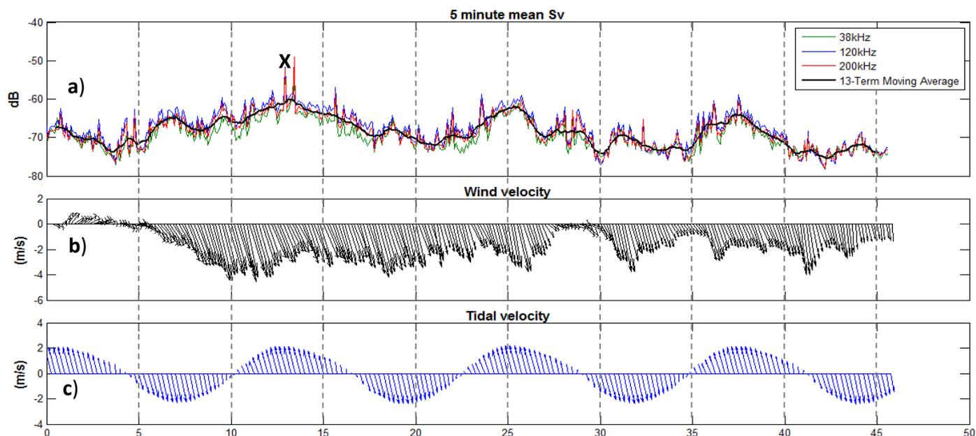
Figure 1. Data from FLOWBEC deployment. Section shows almost 2 days of data from 00:54 on 07/06/2013 with x-axis given in hours. a) Multifrequency mean backscatter variation from 5 minute integrations through entire water column. b) Wind velocity vectors recorded at nearby EMEC operated weather station. c) Tidal velocity vectors from model data.
