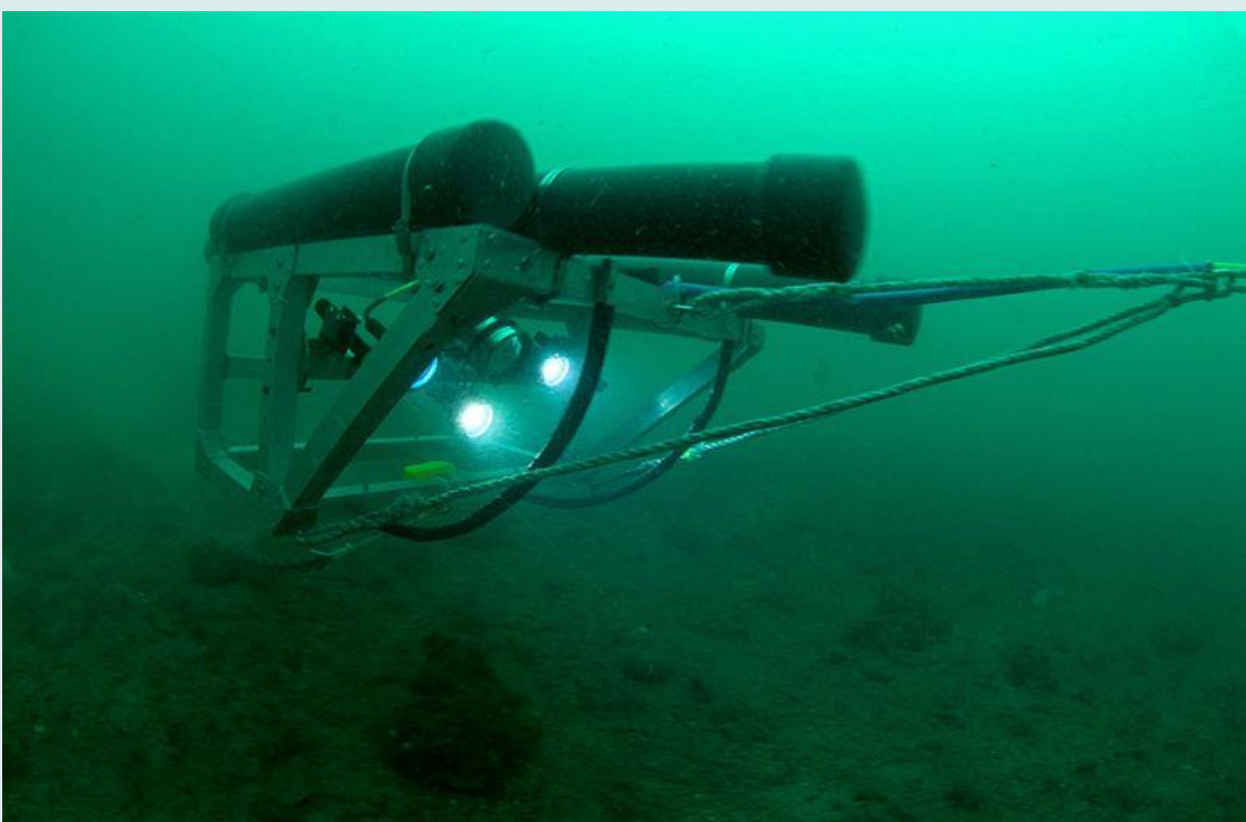
Fig. 2. The towed flying array with high definition video.
