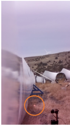
Figure 11. In a second set of experiments, a table tennis ball launcher was used to provide repeatable, low-mass (2.5g) collisions at variable impact velocities. Three impact velocities (7-10 m/s) were used across each of 17 marked 2.5m blade sections, with three replicates of each. Typical measured data is shown for root module and sensor patch.
