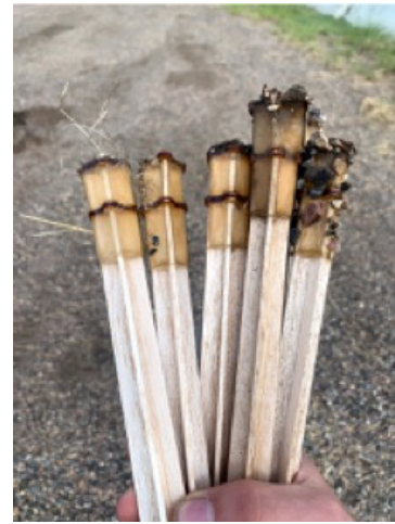
Figure 14. Custom gelatin and balsa wood projectiles designed and built on-site at NREL-NWTC were launched at the blade for surrogate
