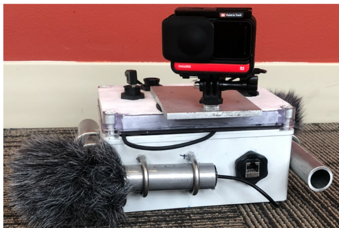
Figure 8. Design and implementation of nacelle-mounted AV unit, including 360° camera module and wideband microphone array for both video and audio capture of nearby birds and bats.
