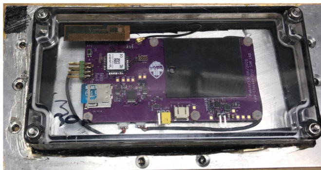
Figure 6. (top) Distributed sensor ‘patches’ on the blade provide localized collision detection to improve system sensitivity. (bottom) The core of the sensor patch is a custom electronics module providing solar energy harvesting and wireless data.
