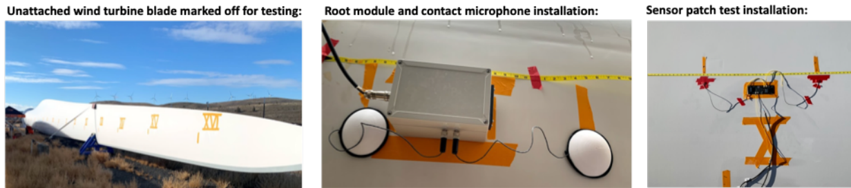
Figure 9. Initial field testing conducted on an unattached wind turbine blade stored on the ground, including installation and validation of all on-blade collision detection and imaging components, following by extensive collision testing using surrogate projectiles and a force-measurement impact hammer. On-blade imager testing, automated image capture of blade strike object, and patch wireless communication range were also validated.
